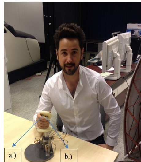
Fig. 6. Integrated micro sensors into a side-stick: a.) micro sensor to measure hearth rate b.) micro sensors to measure skin resistance and body temperature
